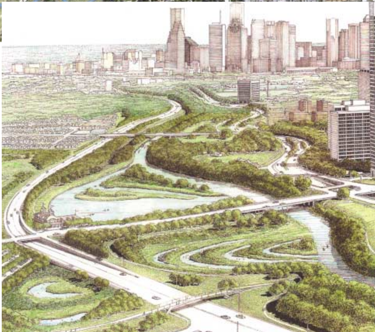
② Reconfiguring the Waugh/Heights and Memorial Drive Intersection (from a cloverleaf to a diamond intersection) will open an additional 20 acres of new park space along the Buffalo Bayou corridor.
